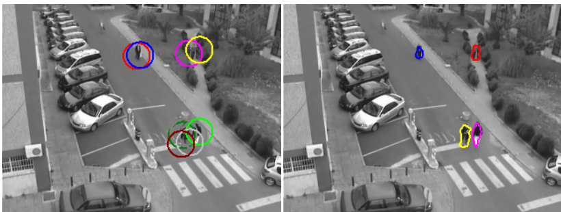
Fig. 2. Pedestrians; 10 initial contours (left) and 4 final estimated contours (right)
