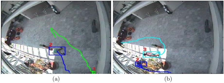
Fig. 3. Plots of trajectory information for (a) Confusing ignoring with approaching. (b) Difficulties when obstacles are in the scene causing mis-classification. Here person 3 has to go round the obstacle to approach person 2. This also illustrates how you may have to watch a sequence for longer to figure out the actual intention of a person. Lines show tracked points from previous timesteps.
